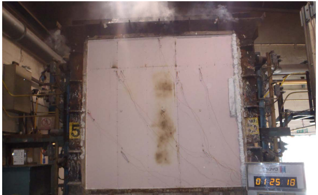
The unexposed face of the test construction after 85 minutes of testing
