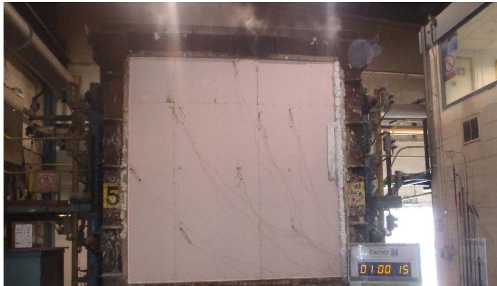
The unexposed face of the test construction after 60 minutes of testing
