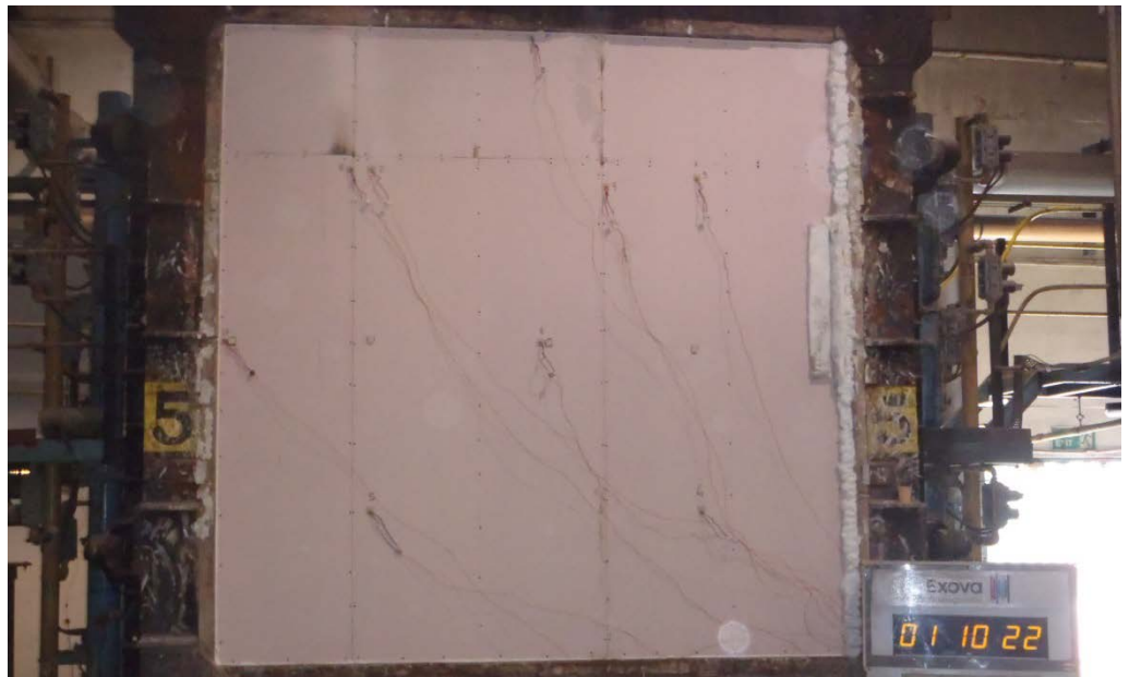
The unexposed face of the test construction after 70 minutes of testing
