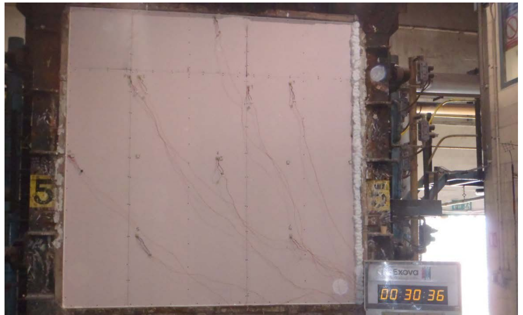
The unexposed face of the test construction after 30 minutes of testing
